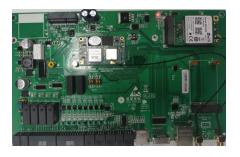
A7 Main Board: backend communication, configuration, display UI& diagnostic log
