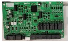
M4 Control Board: output voltage and current control
