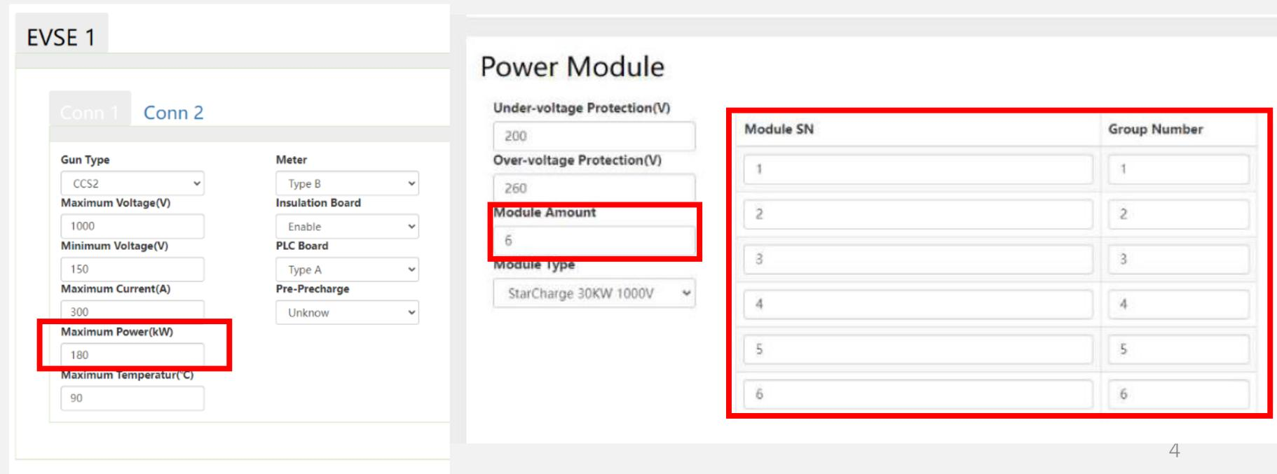
The screenshot displays the configuration interface for EVSE 1, specifically the Power Module settings. The interface is divided into two main sections: EVSE 1 and Power Module.
