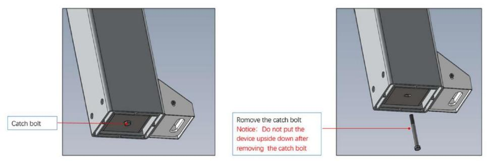
Figure 7 Schematic diagram for removal of catch bolt of wirerope retractor
