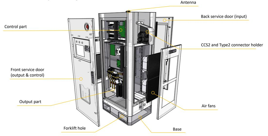
Note: This drawing is based on Jupiter OldID. Its structure is very similar to Jupiter V2, except the position of Type2 socket, emergency button.
